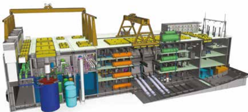
ThorCon 500 MW MSR power plant in ship hull cutaway view ©Thorcon
